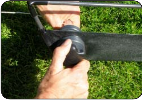
Tighten the leeboard control knob. (Hand tight)
