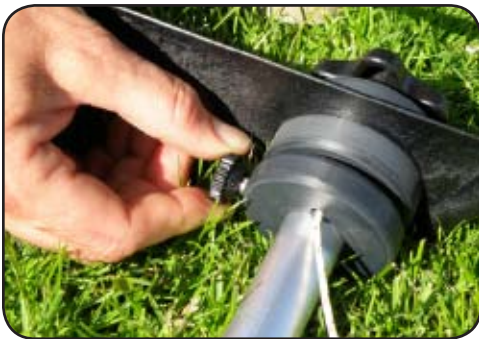
Tighten the shroud ring thumb screw.
